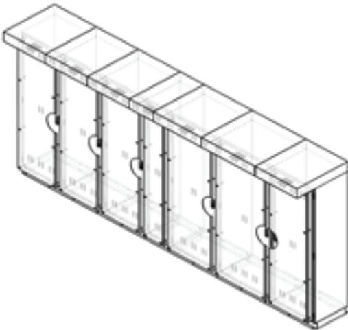
Figure 1: Switchboard for motor control centre of Broome electrical upgrade
